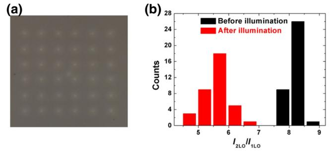
FIG. 3. A pattern of laser-induced modification: a  $6 \times 6$  array with  $5 \mu\text{m}$  spacing on a thin-film ZnTe. (a) Optical image showing illuminated locations. (b) A histogram plot of the  $R_{21}$  ratio before and after illumination.
