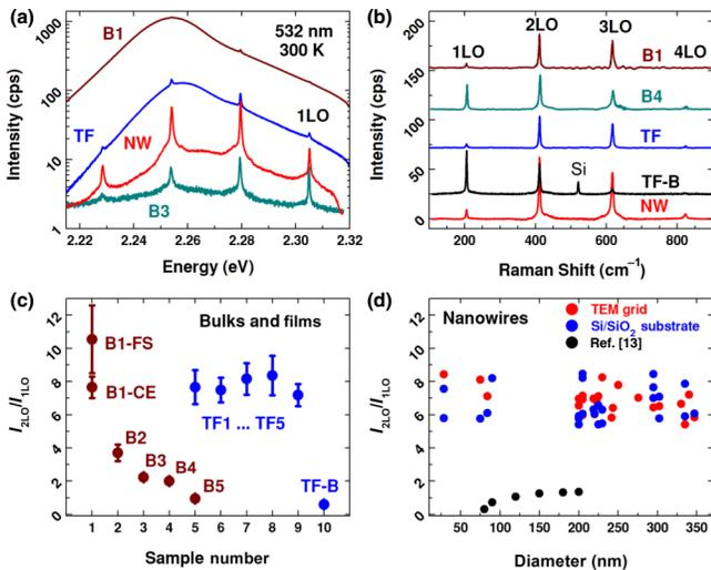
FIG. 1. Representative (a) photoluminescence and (b) resonant Raman spectra at low laser power. (c)  $R_{21}$  values for bulk ZnTe samples (wine) and ZnTe thin films (blue) and (d) for ZnTe nanowires supported by both a TEM grid (red) and SiO<sub>2</sub>/Si substrate (gray).
