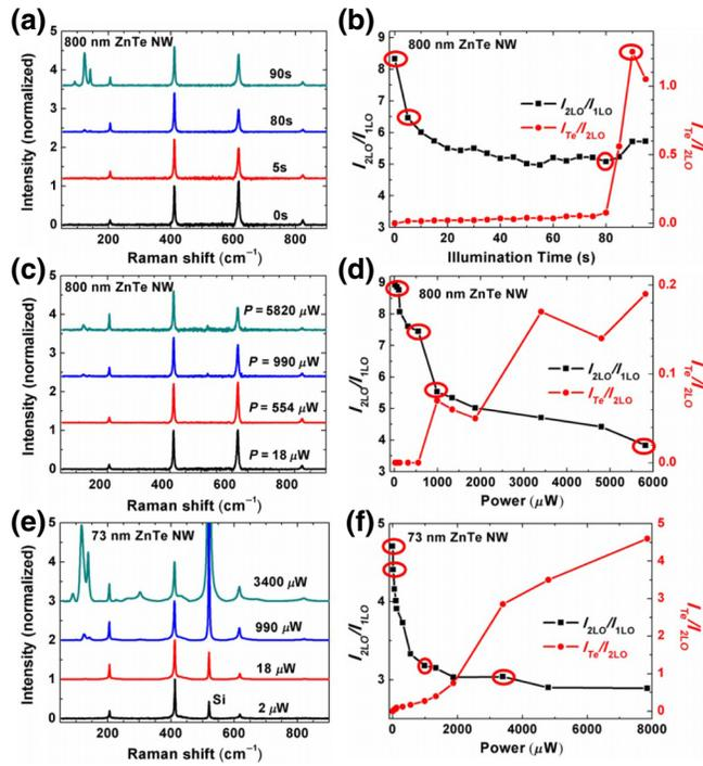
FIG. 2. Laser-induced modifications on Raman spectra of ZnTe NWs. (a),(b): a large NW subjected to repeated illumination of  $750 \mu\text{W}/5 \text{ s}$ , with (normalized) spectra in (a) for selected repeating windows, as marked on (b), and the ratios of  $I_{2\text{LO}}/I_{1\text{LO}}$  and  $I_{\text{Te}}/I_{2\text{LO}}$  at different repeating windows; (c),(d) for the same NW illuminated for 5 s under different powers; (e),(f) a small NW illuminated for 5 s under different powers.
