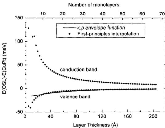
Figure 3. The band edge energies of the conduction and valence band with changing the layer thickness or number of monolayers for an [001] orientational superlattice with fully ordered layers.
