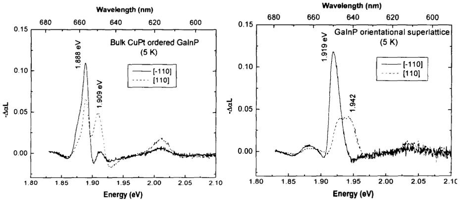
Figure 2. Polarized differential absorption spectra for two ordered GaInP samples: one single variant ordered (left) and one double-variant ordered (right), with nearly the same order parameter and average composition.
