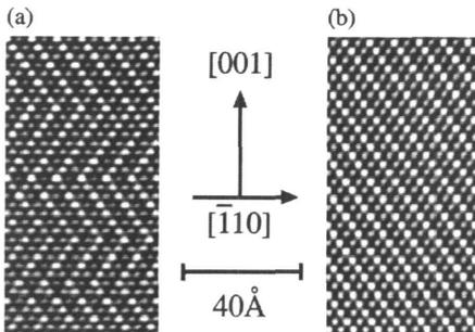
Figure 1. High-resolution cross-sectional TEM pictures of (a) a double-variant ordered and (b) a single-variant ordered GaInP alloys.
