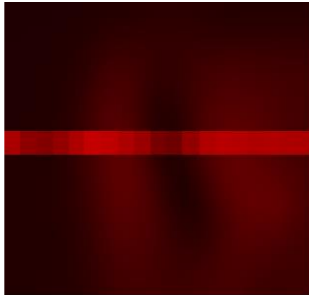
Figure 32: 1-D PL intensity map made with TCSPC system superimposed on 2-D PL map made using LabRam 800 Raman microscope.
