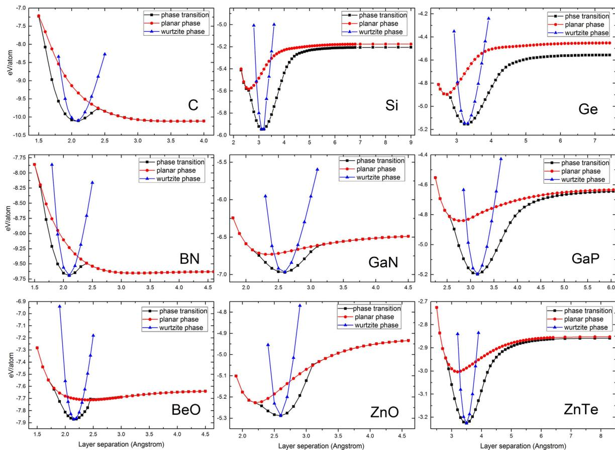
**Figure 2.** Variation of the total energy vs.  $c/2$  (the separation of the bilayer) for three cases. (a) ideal wurtzite structure with a fixed  $u$  parameter (blue), (b) hexagonal planar structure (red), and (c) allowing full relaxation but keeping the  $\overline{AA}$  stacking (black).
