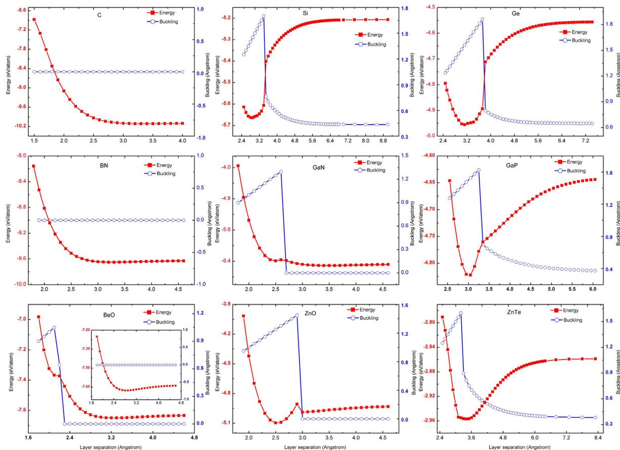
**Figure 4. Phase transition path around NiAs-like structure.** The line with red squares indicates the total energy vs. layer separation and the line with blue circles indicates the buckling height vs. layer separation.
