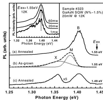
Fig.5. Comparison of the low-temperature PL spectra of the as-grown and annealed GaAs<sub>0.985</sub>N<sub>0.015</sub>/GaAs SQW under different excitation energies. The inset shows the 12 K PL spectra of the annealed sample under different excitation power.
