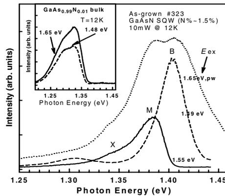
Fig.4. 12 K PL spectra of the GaAs<sub>0.985</sub>N<sub>0.015</sub>/GaAs SQW under different excitation energies. The inset shows the selectively excited PL of GaAs<sub>0.99</sub>N<sub>0.01</sub> bulk sample.
