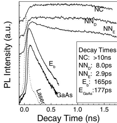
Fig.2. PL decay curves of the  $x=0.1\%$  sample monitored at GaAs PL,  $E_b$ ,  $NN_E$ ,  $NN_D$ , and NC.
