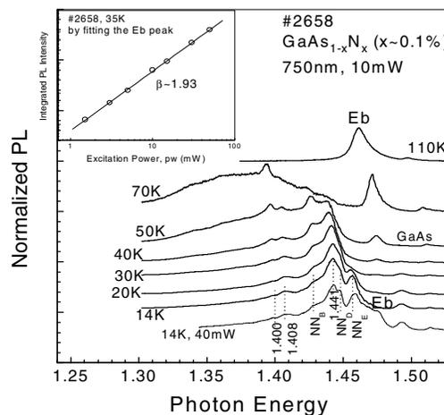
Fig.1. PL spectra of the  $\text{GaAs}_{1-x}\text{N}_x$  sample ( $x=0.1\%$ ) under cw excitation at various temperatures. The inset shows the integrated PL intensity as a function of excitation power.
