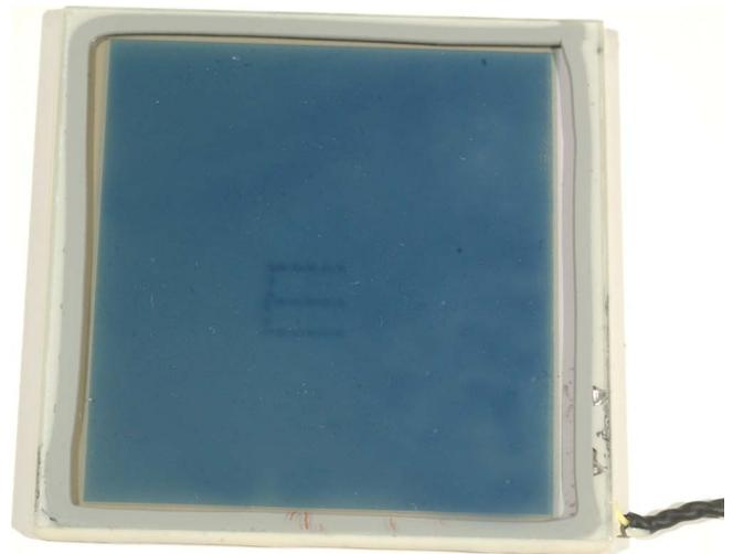
FIG. 1. (Color online) A photograph of a proton-based WO<sub>3</sub> EC device in the colored state, showing a letter E written by an UV laser.
