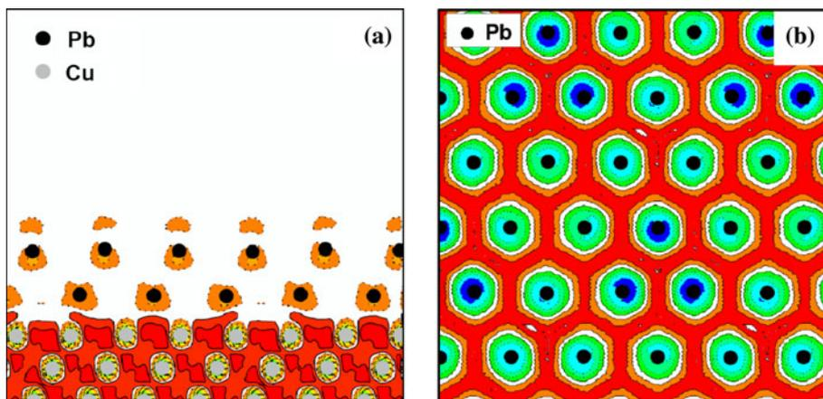
**Fig. 5** **a**  $\Delta\rho_1(\vec{r})$  for the  $(3 \times 3)/(4 \times 4)$  Pb/Cu(111) structure, and the plotted plane is vertical to the Cu(111) surface and along the longer diagonal of the parallelogram pattern (in Fig. 3a); **b** the same as **a**, but the plotted plane is parallel to the Cu(111) surface and
