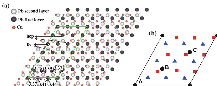
**Fig. 3** **a** Top view of the relaxed  $(3 \times 3)/(4 \times 4)$  Pb/Cu(111) structure, and the *green parallelogram* indicates one super cell. **b** The relative positions of Pb and Cu atoms in Cu(111)  $1 \times 1$  surface cell for the same structure as (a). The *black dot*, *blue triangle* and *red*
