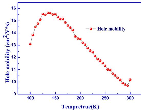
**Figure 6.** Hole mobility as a function of Temperature.
