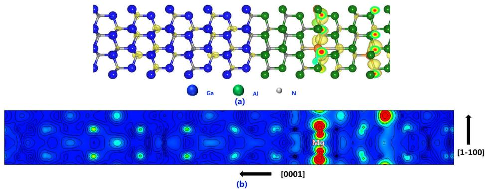
**Figure 2. Distribution of Mg impurity states.** Isosurface charge density plots of Mg impurity states at  $\Gamma$  point in  $\text{Al}_x\text{Ga}_{1-x}\text{N}/\text{GaN}$ . (a) atomic configuration and isosurface charge density of Mg impurity states, (b) isosurface charge density of Mg impurity states in m plane.
