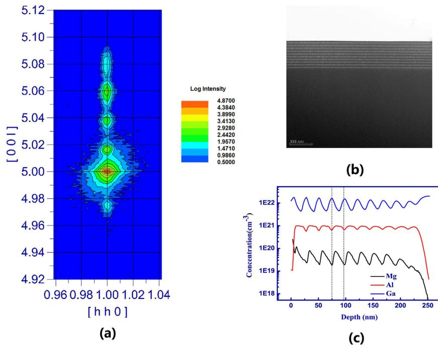
**Figure 4. Structure and crystalline quality of  $\text{Al}_x\text{Ga}_{1-x}\text{N}/\text{GaN}$  sample.** (a) asymmetrical (105) X-ray reciprocal space mapping, (b) TEM image of our  $\text{Al}_x\text{Ga}_{1-x}\text{N}/\text{GaN}$  sample, (c) SIMS depth profiles of Mg for  $\text{Al}_x\text{Ga}_{1-x}\text{N}/\text{GaN}$  sample.
