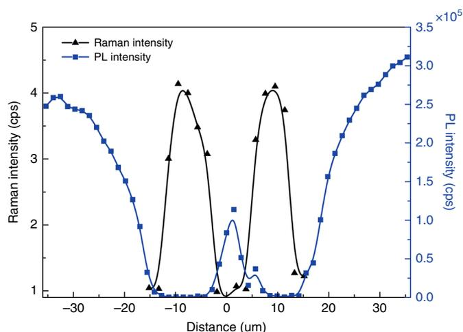
**Fig. 4** Spatial profiles of the PL and  $L_+$  mode intensity measured along a line, shown in Fig. 1b, passing the doublet defect in S2 (at  $5.6 \times 10^4 \text{ W/cm}^2$ )
