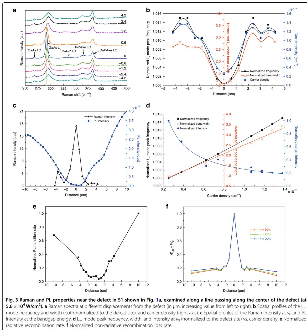
mapping is a generally applicable and effective tool for realizing BDL defect imaging in semiconductors under different sample conditions.
