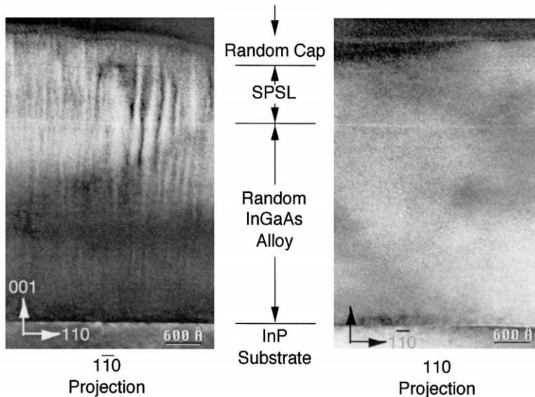
Fig. 1. Dark field images of the  $(\text{InAs})_n/(\text{AlAs})_m$  SPS structure for the  $[1\bar{1}0]$  and  $[110]$  projections. The left side of the figure shows the lateral contrast variation due to showing lateral composition modulation but not in the orthogonal projection shown on the right side.
