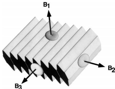
Fig. 3. Schematic drawing showing the lateral spatial variation of the band-gap energy from the CM wave. The three principal orientations of the magnetic field are  $B_1$ ,  $B_2$ , and  $B_3$  where  $B_1$  is the growth direction. The “donut” shapes represent the plane of the aligned exciton orbits.
