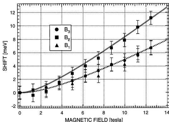
Fig. 4. Diamagnetic shifts for the CM SPS structure. The magnetic field orientations for the three shifts correspond to the alignments shown in Fig. 3. The best-fit curves of Eq. (1) to the data yield reduced masses  $\mu(B_2) = 0.042$  and  $\mu(B_1) = \mu(B_3) = 0.056$ .
