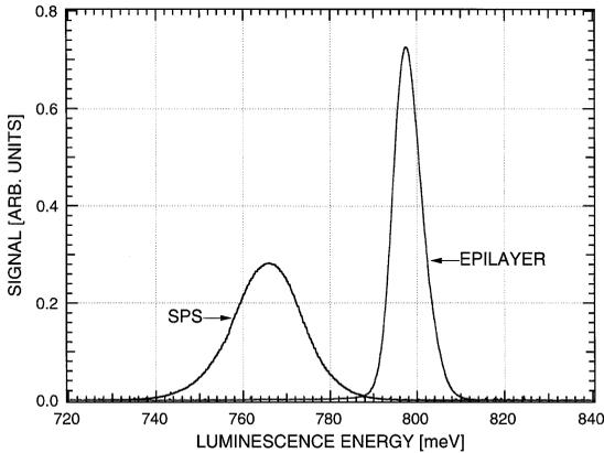
Fig. 2. Two 1.4 K zero-field PL spectra for the CM SPS structure (left) and the InGaAs-epilayer (right).
