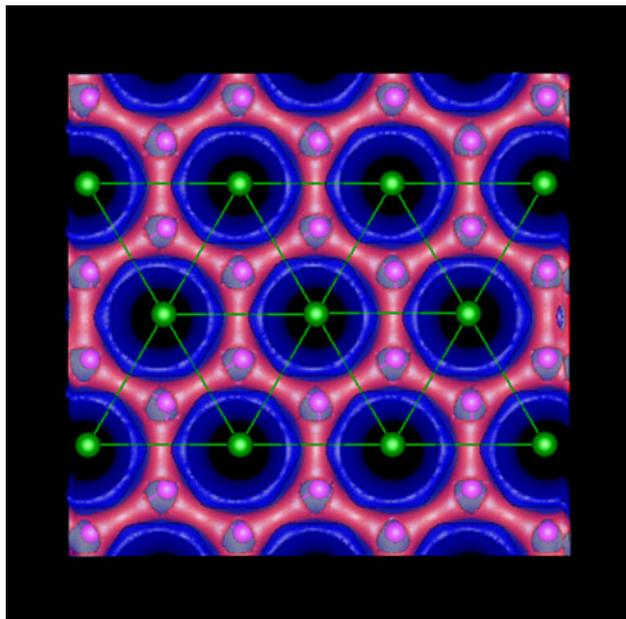
**Fig. 1** The atomic structure of graphene/Si superlattice, with Si atoms on top, projected onto the graphene plane, overlaid with two contour plots of the total charge density. The contour of the 80% maximum (*red*) reveals the charge distribution on graphene, and the 20% contour (*blue*, drawn with 40% opacity) shows the charge distribution on the Si sheet
