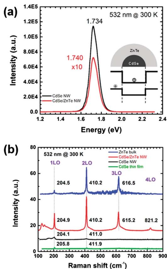
Fig. 3 Optical characterization of CdSe nanowires and CdSe/ZnTe core–shell nanowires. (a) Photoluminescence spectrum of a representative CdSe nanowire and CdSe/ZnTe core–shell nanowire. Inset: type-II heterojunction diagram of a CdSe/ZnTe core/shell structure. (b) Raman spectra of a representative CdSe nanowire and CdSe/ZnTe nanowires with spectra of bulk ZnTe and a CdSe thin film for reference.
