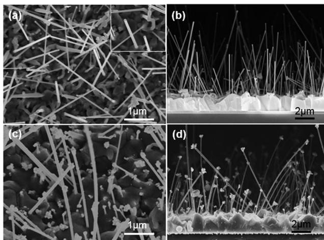
**Fig. 1** CdSe and CdSe/ZnTe core-shell nanowire morphologies observed in SEM. CdSe nanowires grown on a silicon substrate by thermal evaporation observed from (a) top- and (b) cross-sectional views. CdSe/ZnTe nanowires imaged from the (c) top- and (d) cross-sectional views. Note the increased diameter from the shell and the nanoparticles on the tip and shell surface.
