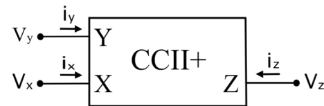
Fig. 1. Basic CCII+ current conveyor voltages and currents.
