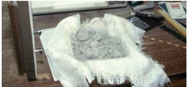
Figure 5.13. Microwave test to determine w/cm ratio of mixture in the field
