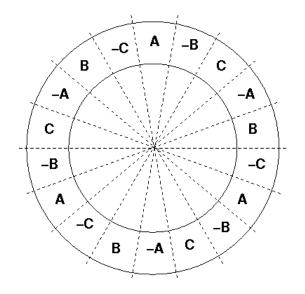
What is the physical angle between any one of the A coils and the nearest –A coil (Note that –A coils would contain a current flowing in the opposite direction)? What is the electrical angle between then? What is the physical angle between any one of the A coils and the nearest B coil? What is the electrical angle between them? What is the physical angle between any one of the A coils and the nearest B coil? What is the electrical angle between them? What is the electrical angle between them?
