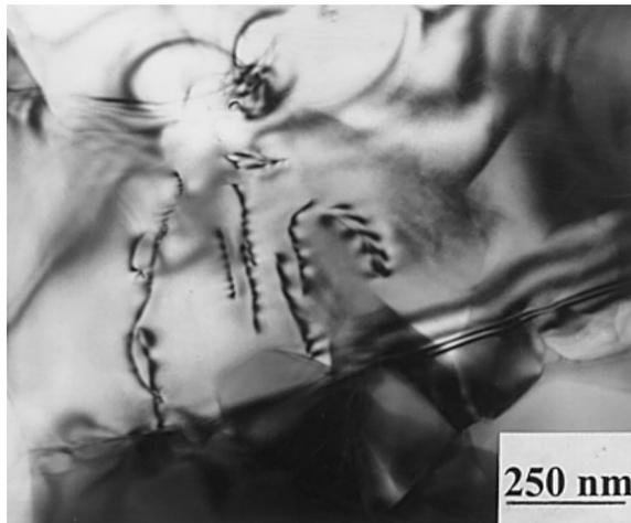
Fig. 13. Dislocations starting from contacting point of two silicon nitride grains. Trace of strain whorl can also be seen at the back end of a dislocation in the lower left corner of the micrograph.
