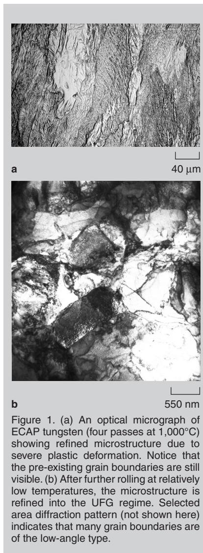
Figure 1. (a) An optical micrograph of ECAP tungsten (four passes at  $1,000^\circ\text{C}$ ) showing refined microstructure due to severe plastic deformation. Notice that the pre-existing grain boundaries are still visible. (b) After further rolling at relatively low temperatures, the microstructure is refined into the UFG regime. Selected area diffraction pattern (not shown here) indicates that many grain boundaries are of the low-angle type.
