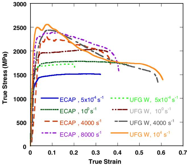
Fig. 3. True stress–strain curves of the ECAP W and the ECAP + CR (UFG) W, under uni-axial quasi-static, and dynamic (Kolsky bar) compressive loading. All the samples are rectangular with square loading faces. The quasi-static tests used strain rates  $\sim 10^{-4}$ – $10^0$   $s^{-1}$  (MTS hydro-servo system). For the dynamic testing, the strain rate was determined by the projectile mass and the pressure, as well as the prescribed strain level.
