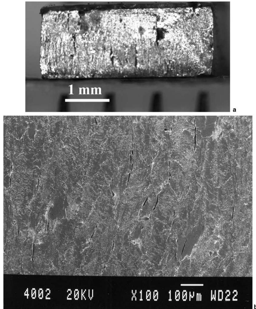
Fig. 4. (a) Post-mortem optical micrograph of dynamically loaded ECAP W (loading is vertical), showing cracks along the loading axes. (b) SEM micrograph of the same sample as (a) showing microcracks approximately parallel to the loading axis (vertical).
