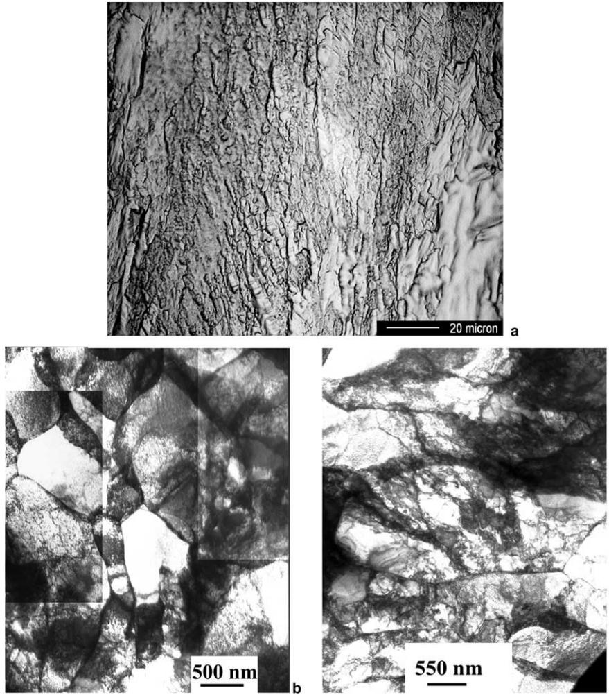
Fig. 1. Optical micrograph (a) of a W sample after four passes of ECAE at 1000 °C. Compared to the original coarse grain (~40 μm) microstructure (not shown here), the refinement of the microstructure is apparent. Transmission electron micrographs of SPD-processed (ECAP + rolling) UFG W (b, c), showing grains and dislocation cell structures refined to sizes of the order of 500 nm. Selected area diffraction (not shown here) shows the presence of both large angle and small angle grain boundaries.
