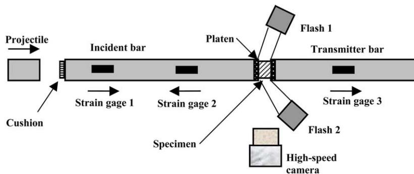
Fig. 2. Schematic of experimental setup for Kolsky bar compressive test with a high-speed camera synchronized with the system. Strain gages 1, 2, 3 are used for the high-speed camera, the incident/reflected and transmitted waves, respectively. The platens are a set of impedance-matched tungsten carbide disks collared with Ti-6Al-4V for the protection of the bars.
