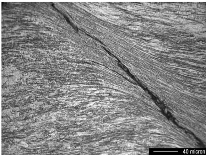
Fig. 6. Morphology of ASB and crack as revealed by chemical etching. Flow lines are clearly observed.
