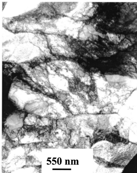
FIG. 1. Transmission electron micrographs of SPD-processed UFG-W, showing grains and dislocation cell structures refined to sizes of the order of 500 nm.
