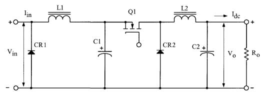
Figure 21-D1. Typical Buck Type Switching Converter.
