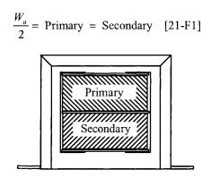
Figure 21-F2. Transformer Window Allocation.
