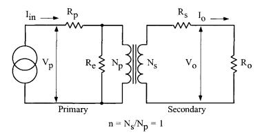
Figure 21-F1. Transformer Circuit Diagram.
