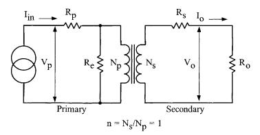
Figure 21-B1. Isolation Transformer.
