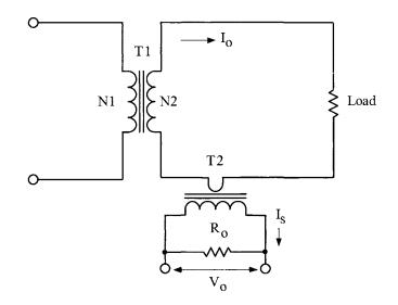
Figure 16-1. Simple, Secondary AC Current Monitor.
