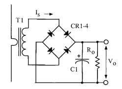
Figure 16-9. Current Monitoring Transformer with dc Output.
