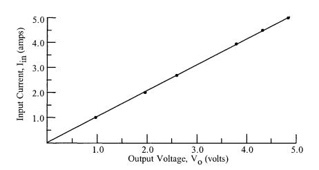
Figure 16-10. Current Transformer, Input Current versus Output Voltage.
