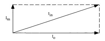
Figure 16-4. Input Current Iin Phase Relationship Diagram.
