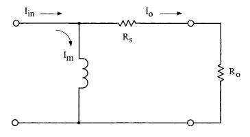
Figure 16-3. Input Current-Output Current Relationship.
