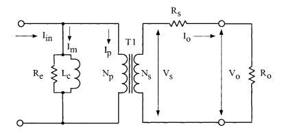
Figure 16-2. Simplified, Equivalent Circuit for a Current Transformer.
