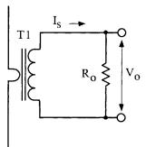
Figure 16-6. Current Transformer, T1, used to Monitor Line Current.
