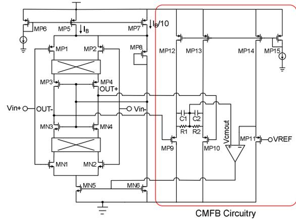
Fig. 3. Configuration of the complementary-input telescopic amplifier.
