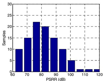
Fig. 7. Monte Carlo simulation of PSRR (100 runs).
