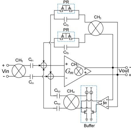
Fig. 1. Configuration of the proposed chopper-stabilized amplifier.
