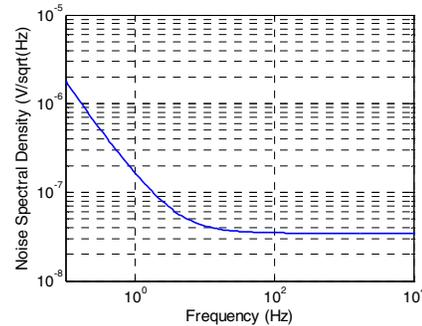
Fig. 5. The simulated input-referred noise spectrum of the chopper stabilized amplifier.
