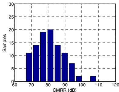
Fig. 6. Monte Carlo simulation of CMRR (100 runs).
