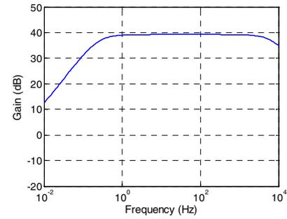
Fig. 4. The simulated transfer function of the chopper stabilized amplifier.
