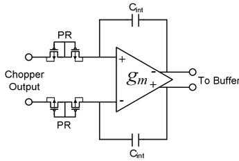
Fig. 2. Configuration of the pseudo-resistor based integrator.
