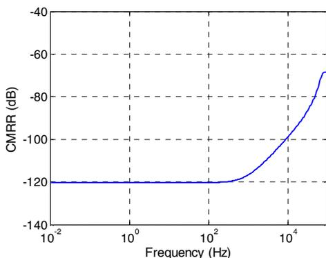
Fig. 5. The simulated CMRR of the instrumentation amplifier.
