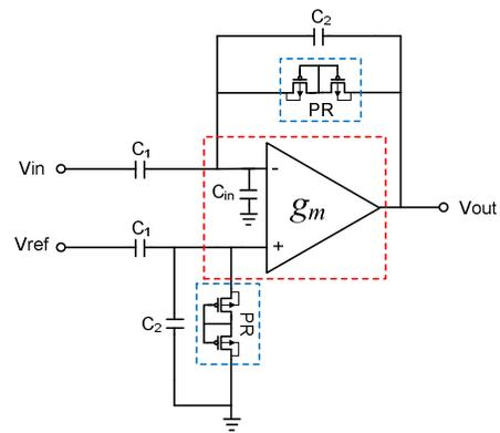
Fig. 1. Configuration of the capacitive-feedback bio-potential amplifier.
