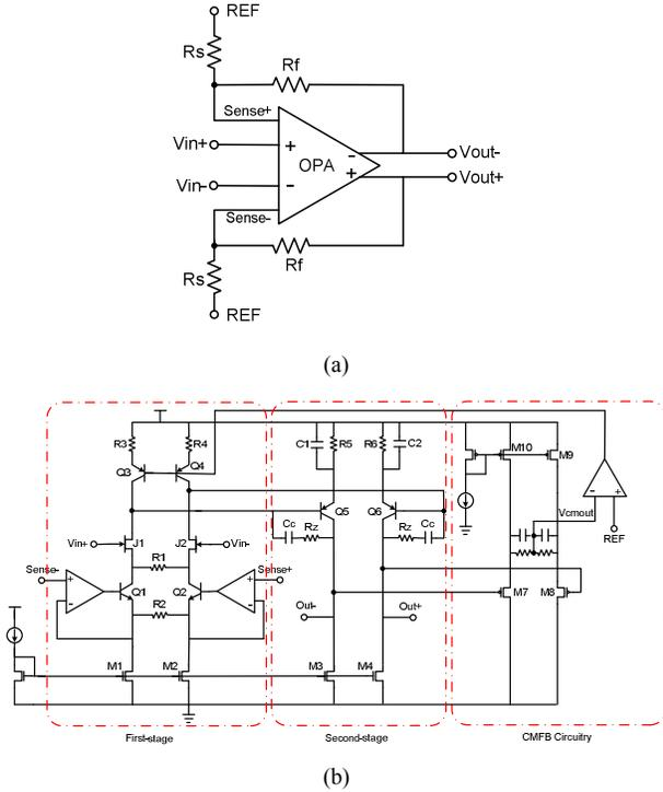
Fig. 2. (a) The configuration of the proposed instrumentation amplifier. (b) The schematic of the operation amplifier (OPA) with sensing terminals.
