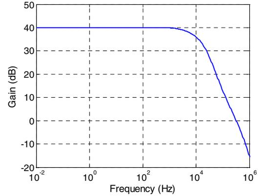
Fig. 3. The simulated transfer function of the instrumentation amplifier.
