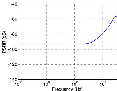
Fig. 6. The simulated PSRR of the instrumentation amplifier.
