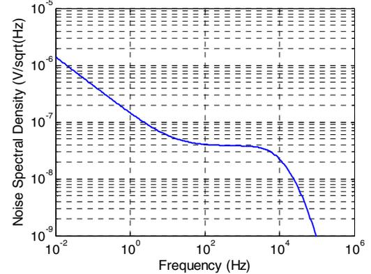
Fig. 4. The simulated input-referred noise spectrum of the amplifier.
