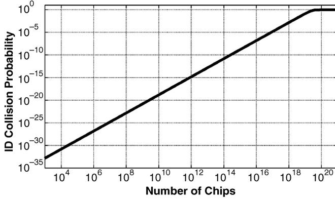
Fig. 3. Probability of ID collision versus number of chips for a randomly assigned 128-bit chip ID.
