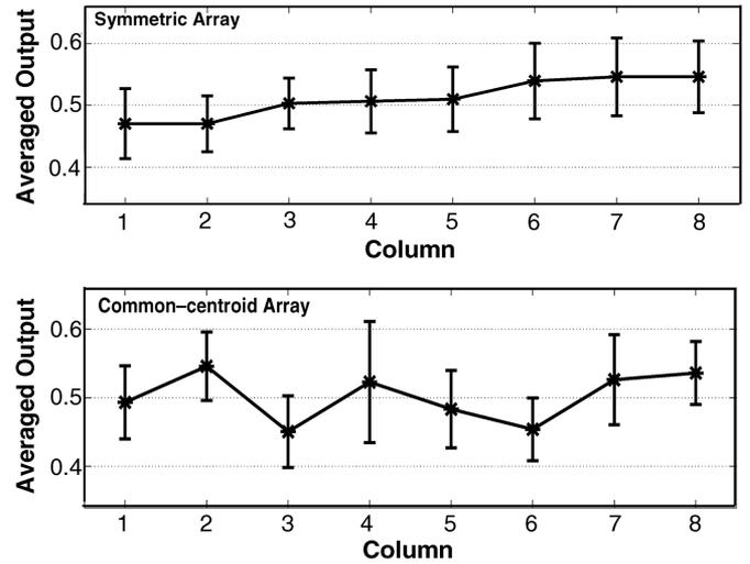
Fig. 13. Averaged output of all ID columns showing gradient effects.
