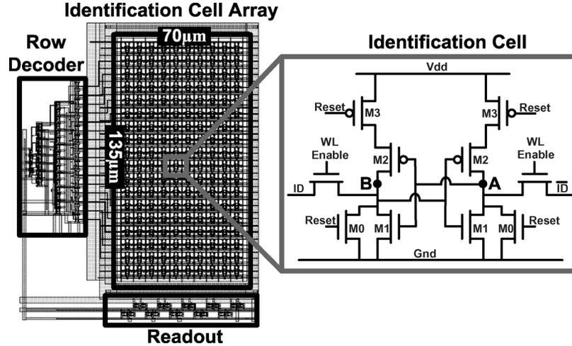
Fig. 1. Simplified ID generator schematic and layout of ID array with perimeter dummy cells.
