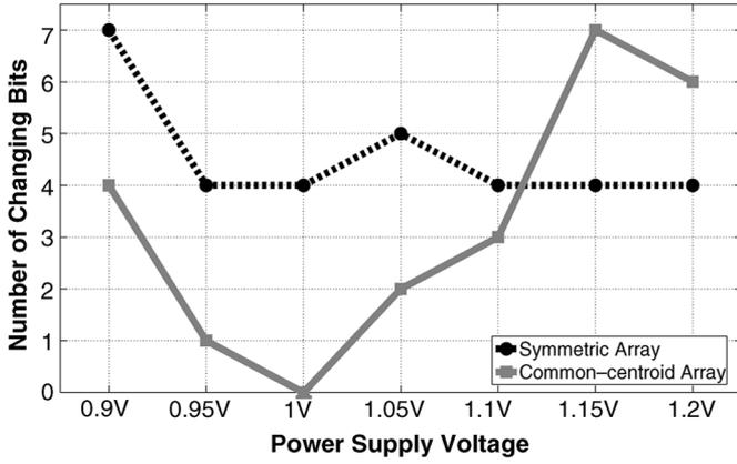
Fig. 10. Measured supply dependency of chip ID.
