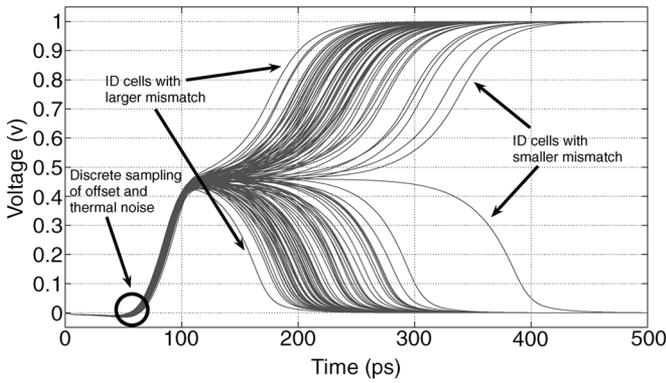
Fig. 2. Monte Carlo simulation of a 128-bit ID cell generator.
