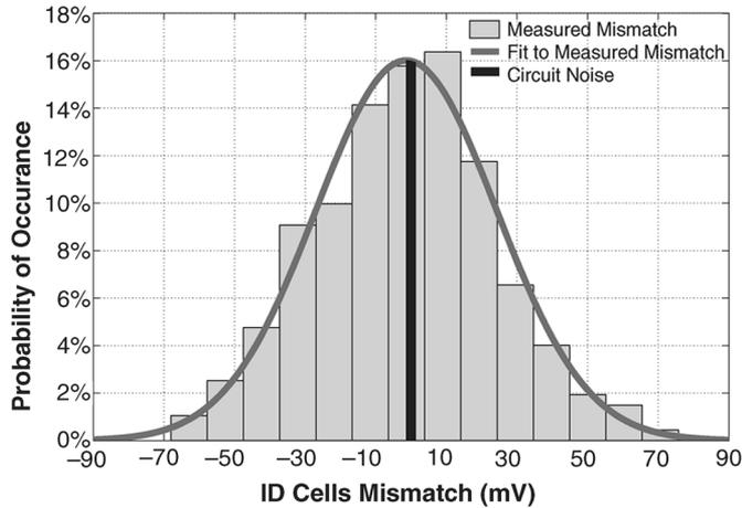
Fig. 5. Measured ID cell mismatch distribution. The calculated RMS circuit noise is annotated with the black zero-mean stripe.
