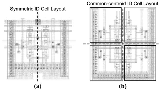
Fig. 6. Layout of a symmetric ID cell and a common-centroid ID cell.
