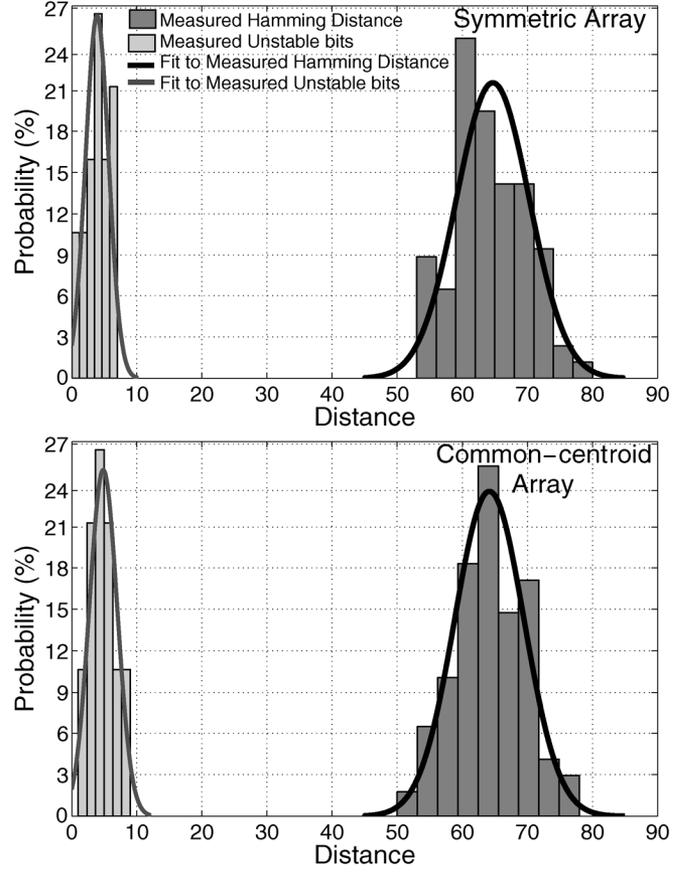
Fig. 9. Measured Hamming distance and unstable bits for both ID generators.
