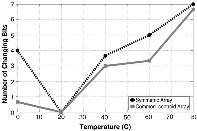
Fig. 11. Measured temperature dependency of chip ID.
