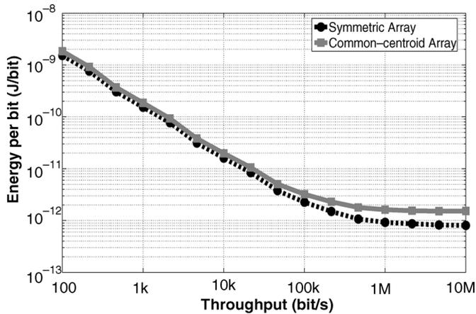
Fig. 14. Energy per bit (J/b) versus throughput (b/s). Below approximately 100 kb/s, static leakage dominates the power consumption.
