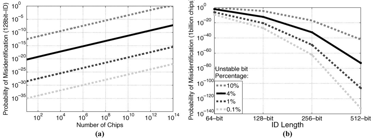
Fig. 4. (a) Probability of chip misidentification versus number of die. (b) Probability of chip misidentification as a function of ID length.
