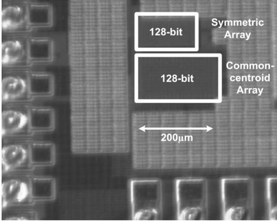
Fig. 7. 0.13  $\mu\text{m}$  CMOS chip micrograph.
