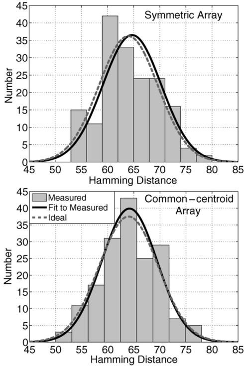
Fig. 8. Measured and ideal Hamming distance for both ID generators.
