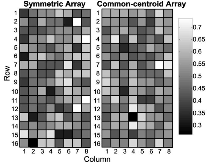
Fig. 12. Averaged ID generator output showing spatial dependency.
